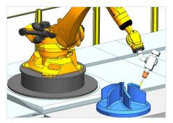
Program robots to machine large parts and to automate machining tasks typically performed manually, such as polishing, trimming and deburring.
