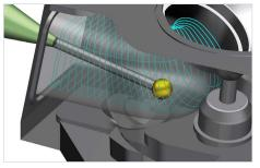
Tube machining streamlines programming of complex hollow regions typically found in manifolds, cylinder head ports and shrouded impellers.
