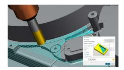
Adaptive milling's smooth patterns enable deep cuts at high machining speeds while managing the tool load, which accelerates machining and extends tool life.
