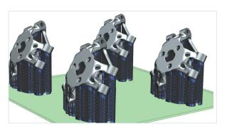
NX's advanced 3D printing preparation tools assist with placing, orienting, and supporting parts in the build tray in the most efficient manner possible.
